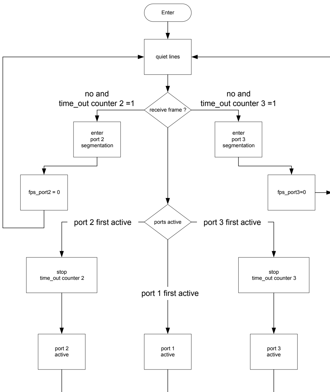
Figure G.7 — Main switch state machine
